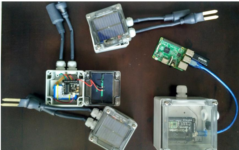
FIGURE 3. Nodes and gateway used in the experiment.
