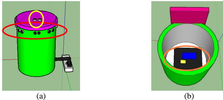
FIGURE 2. Garbage bin proposed in this research (a) ultrasonic sensors placement
