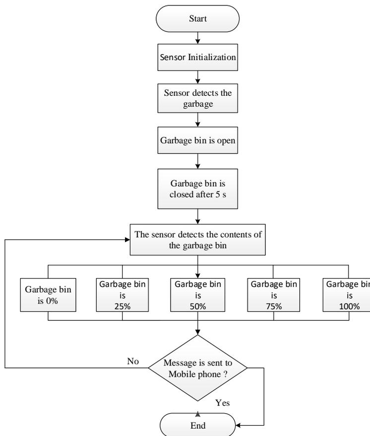
FIGURE 3. Flowchart of the garbage bin monitoring system
