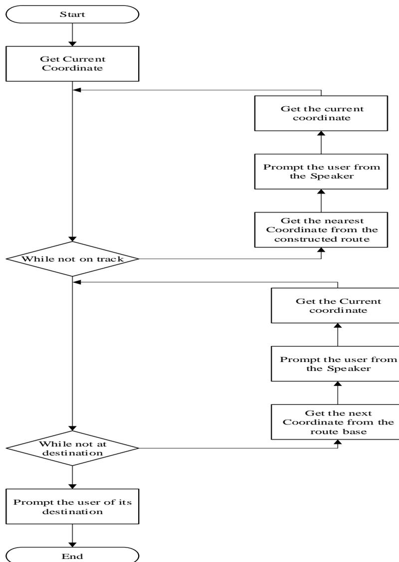
FIGURE 5. Flow Chart of Navigation Module
