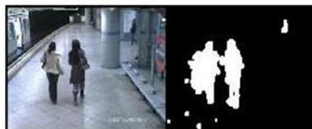
Figure 1. a) current frame b) result of temporal differencing
