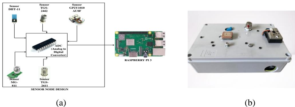
FIGURE 1. (a) Block Diagram of Air Quality Monitoring System Design, (b) Hardware
