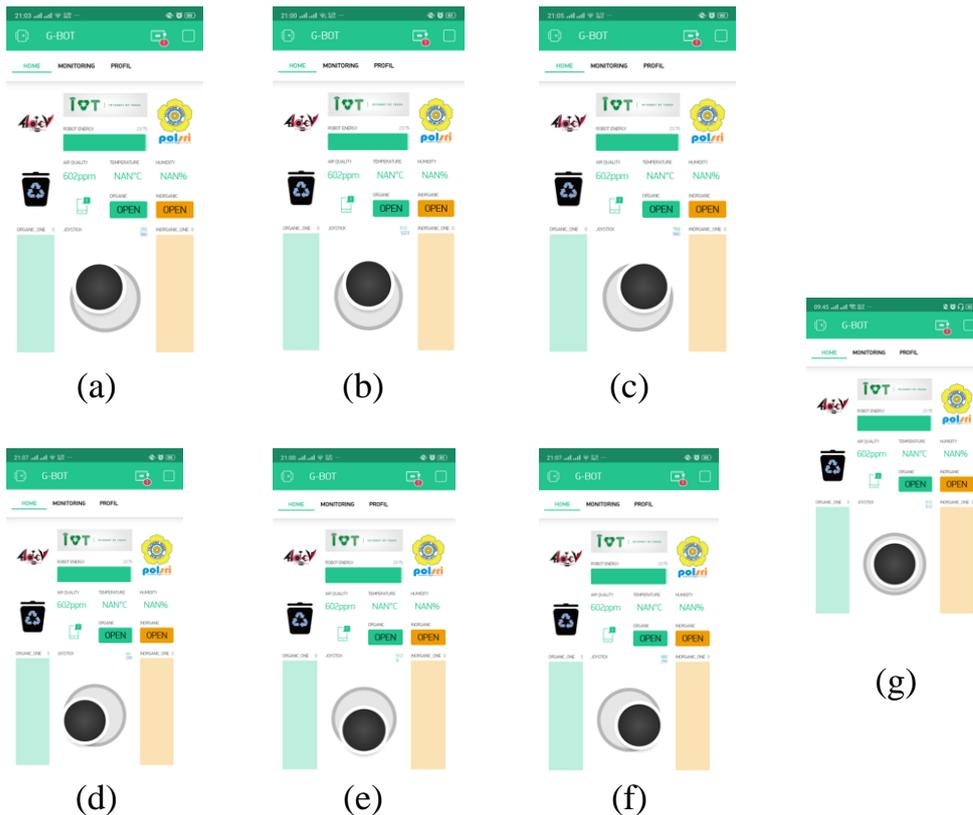
FIGURE 4. The position of the G-Bot movement control button, (a) Left Oblique Forward, (b) Forward, (c) Right Oblique Forward, (d) Left Oblique Backward, (e) Backward, (f) Right Oblique Backward, (g) Stop
