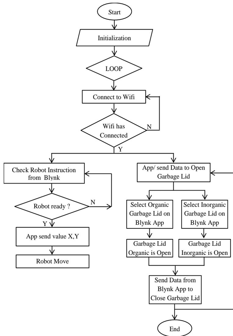
FIGURE 3. Flowchart of the G-Bot Moving
