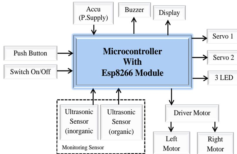
FIGURE 1. G-Bot Block Diagram
