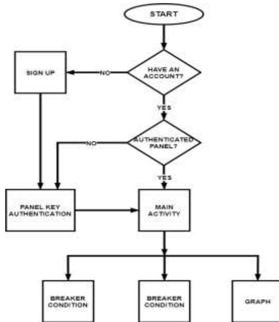
FIGURE 5. IMCB Software Application Activity Diagram
