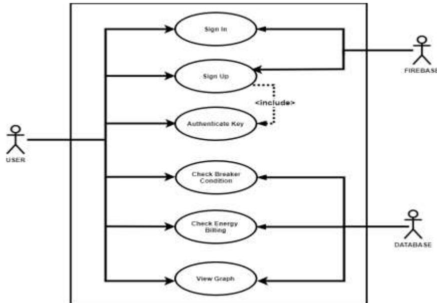
FIGURE 4: System Software Use Case Diagram
