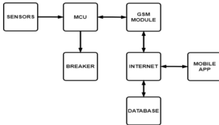
FIGURE 2. IMCB System Block Diagram
