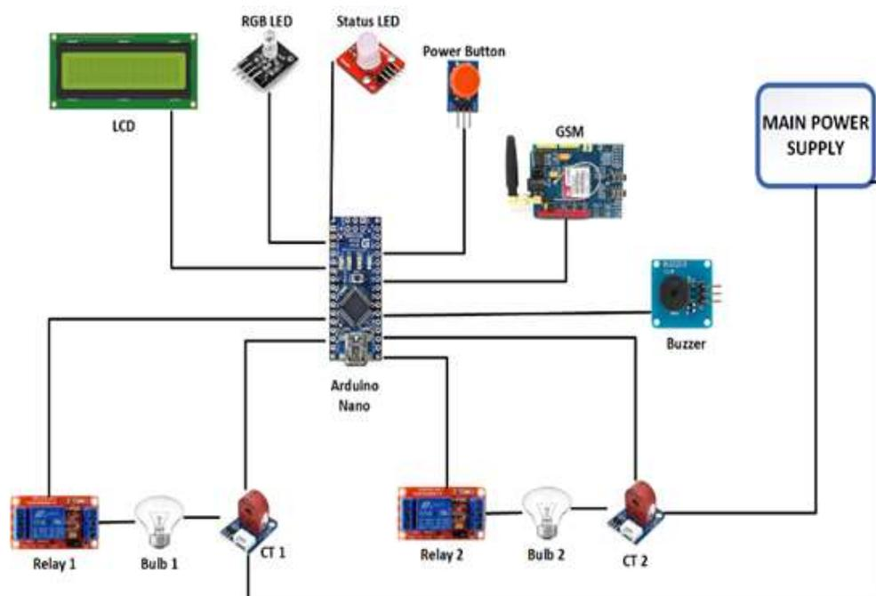
FIGURE 7. Proposed IMCB System Test Diagram
