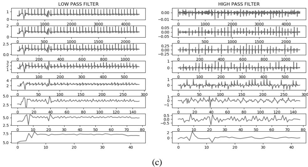
FIGURE 2. (a) Signal before denoising process. (b) Signal after denoising process. (c) Decomposition of 8 Level Low Pass Filter and High Pass Filter of Signal Denoising
