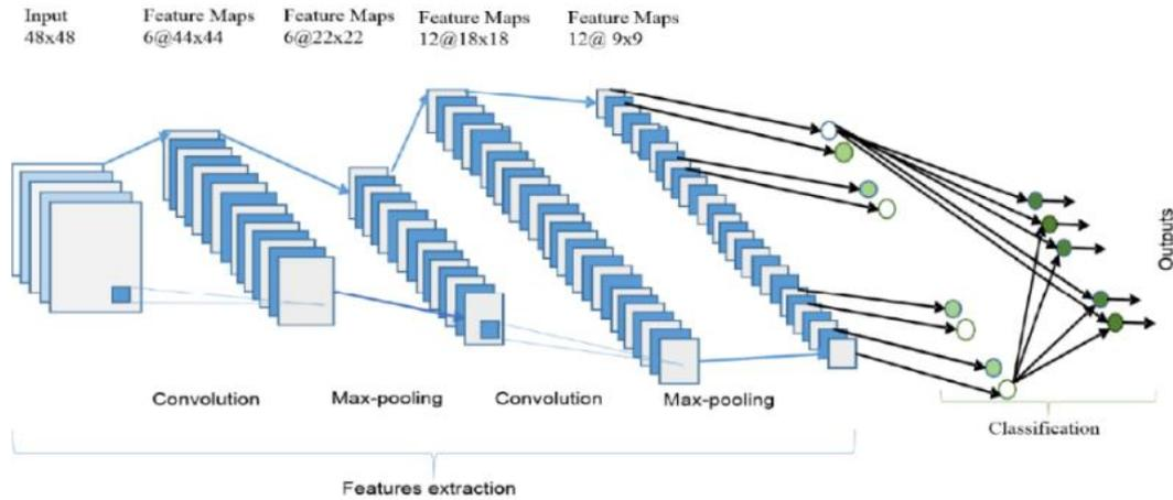
FIGURE 2. CNN Process
