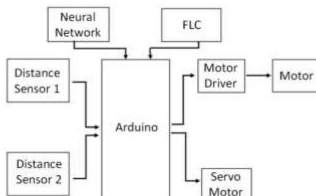
FIGURE 1. Diagram block of FLC and NN application in this study.
