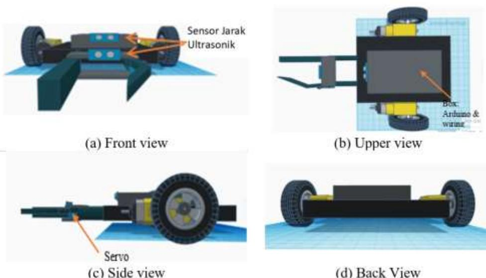
FIGURE 2. The mechanical design of goods transport mobile robot
