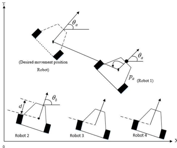
FIGURE 2. Multi-robot System Formation Model
