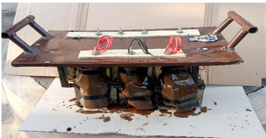
FIGURE 2. Three Phase distribution transformer
