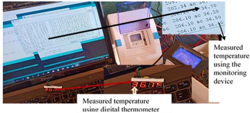
FIGURE 5. Experimental setup for temperature calibration
