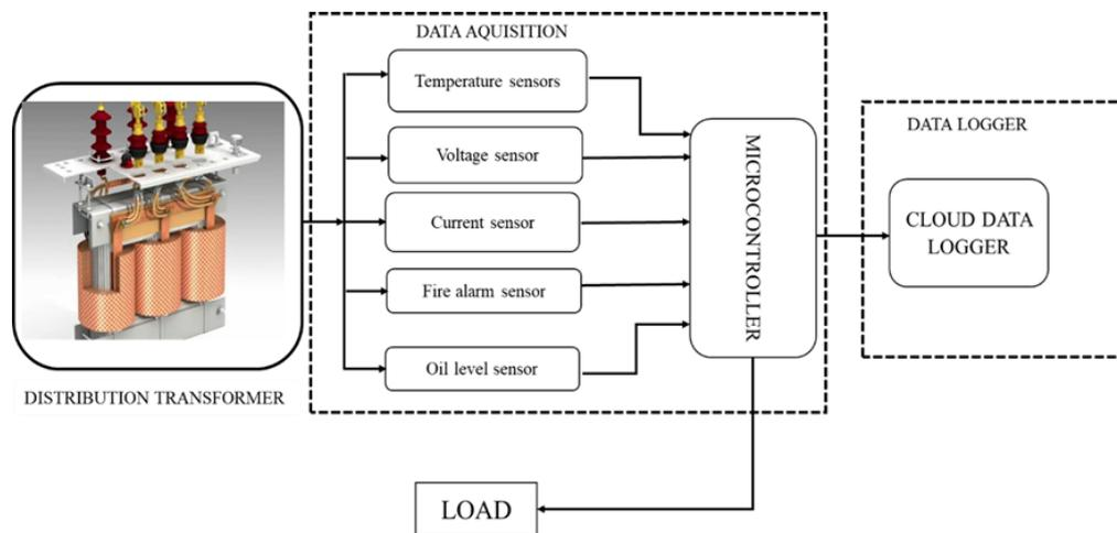
FIGURE 1. Cloud-based condition monitoring of distribution transformer
