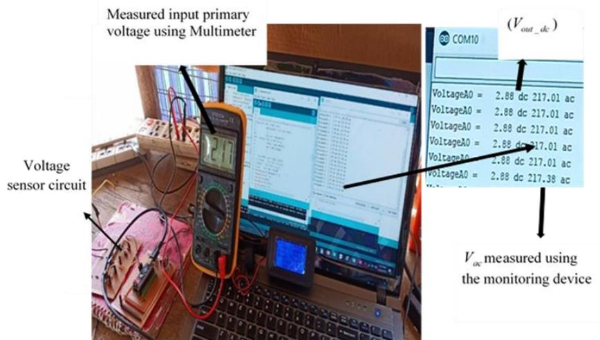
FIGURE 3. Experimental setup for voltage calibration
