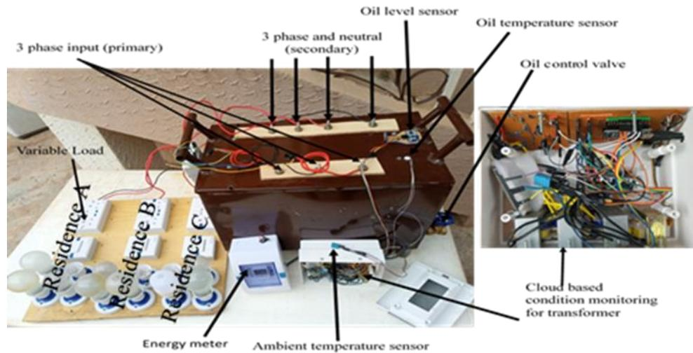
FIGURE 11. Experimental setup for cloud-based condition monitoring device
