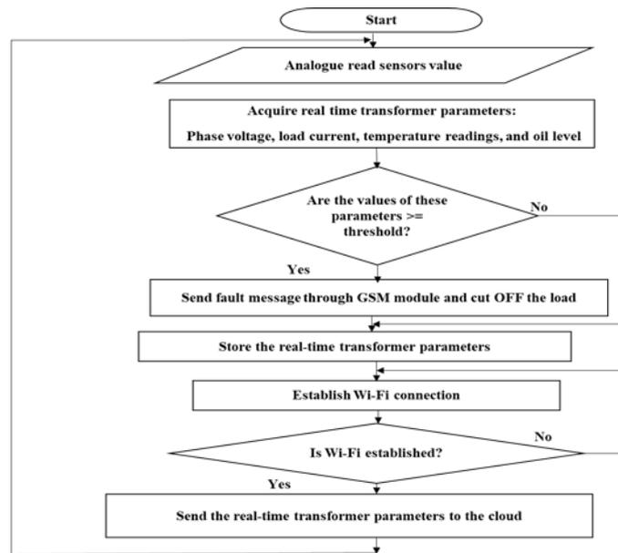
FIGURE 9. Algorithm flow chart for the monitoring device
