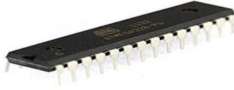
FIGURE 7. ATmega328P microcontroller
