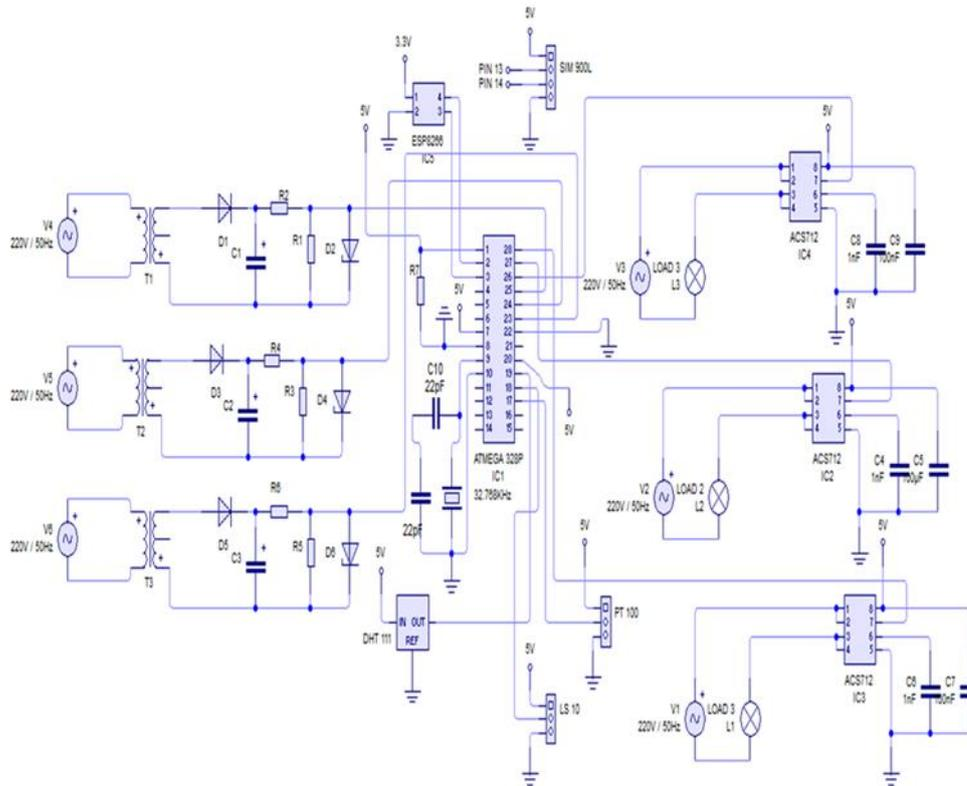
FIGURE 10. Circuit diagram of the monitoring device
