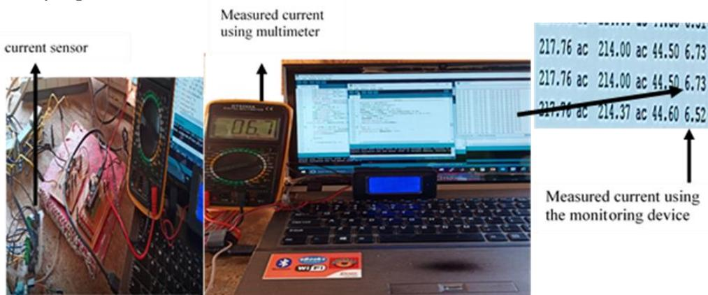
FIGURE 4. Experimental setup for current calibration
