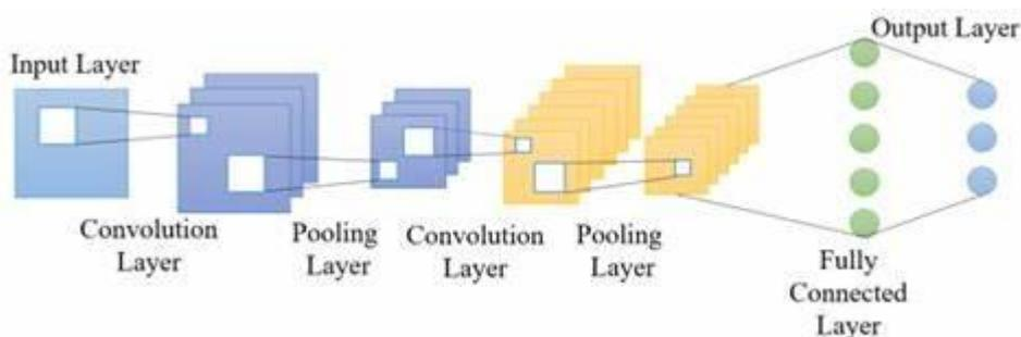
FIGURE 2. CNN architecture
