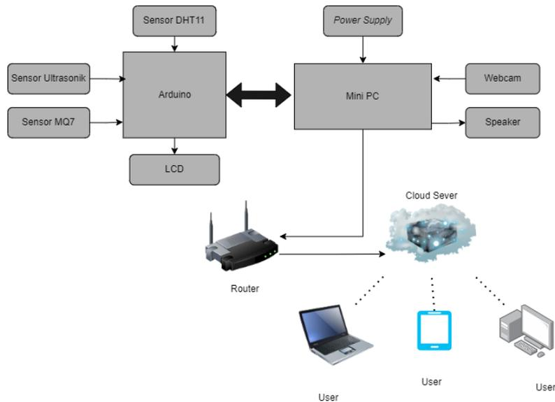
FIGURE 3. Block Diagram of Monitoring System
